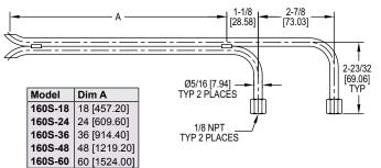
The Series 160S "S" Type Stainless Steel Pitot Tubes are designed specifically for flow measurement of dirty, particulate laden air or gas streams typical in smoke stack and other environmental testing. Total and static pressure tubes are precisely aligned and welded together every 6 inches for maximum accuracy, strength, and long term durability. Permanent mount (PM) models include a 1" welded stainless steel sleeve and adjustable compression fitting with 1" MNPT mounting threads.
